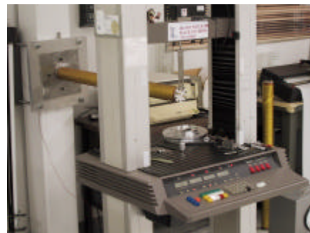
Figure 13. Bending Test Setup
