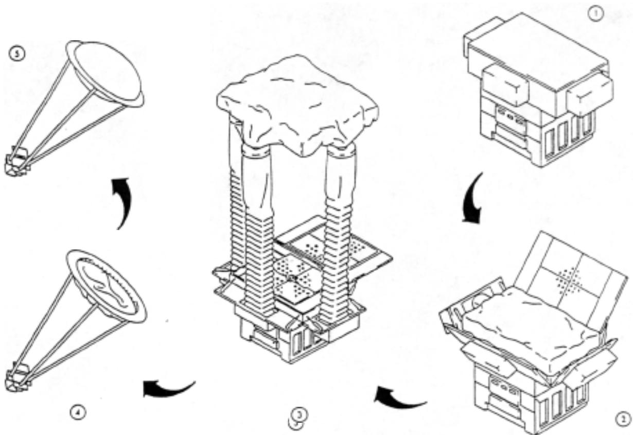
Figure 3. Antenna Deployment Sequence
