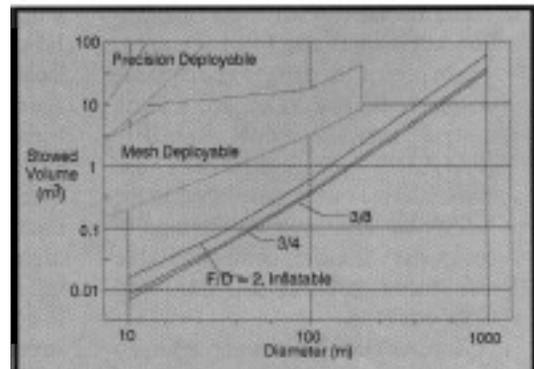
Fig. 4. Inflatables can generally be stored in volumes several orders of magnitude less than needed by competing structures.
