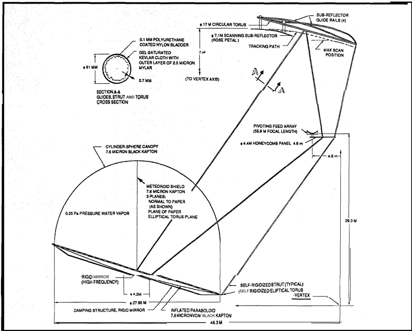
Fig. 7. Application of a large inflatable reflector for an Earth sciences Geostationary Platform.
