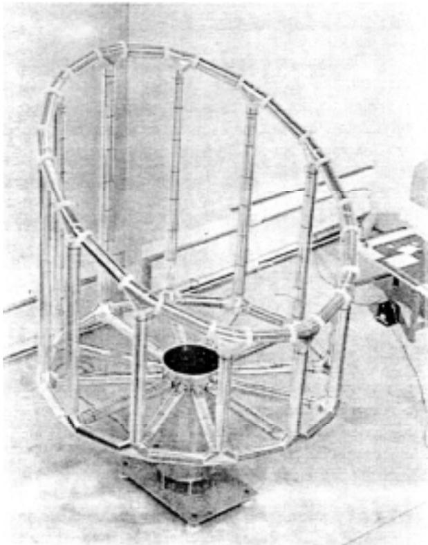
Figure 6. Telescope Sun Shade Support Structure
