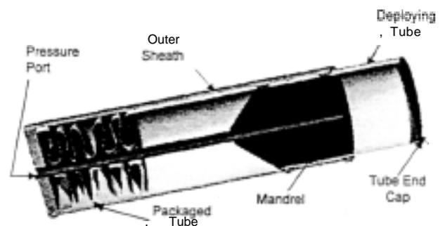
Figure 16. Fan Fold Method
