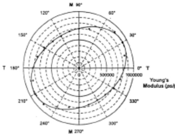
Figure 20. Youngs Modulus for 1/2 Mil Mylar as a Function of Angular Orientation
