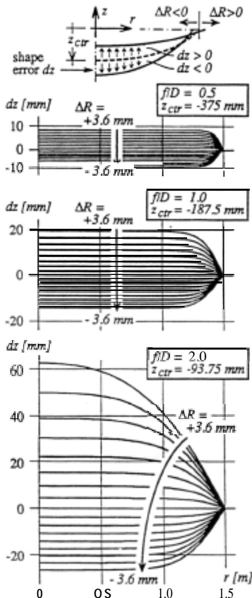
Figure 23. Effect of In-Edge Displacement on Deflected Shape
