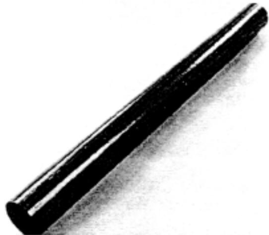
Figure 13. Carbon Fabric Impregnated with Thermally Activated Epoxy
