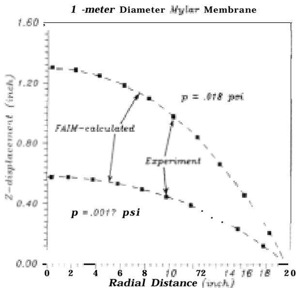
Figure 21. Measure Mylar Profile from Figure 19 Test Article. Membrane Center Stress Equals 636 psi and 3076 psi
