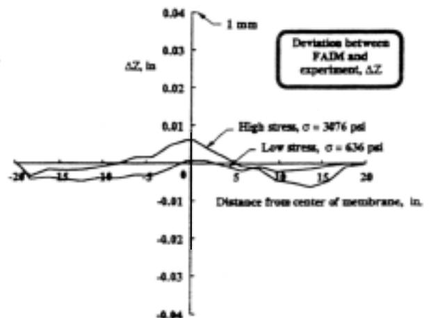
Figure 22. Deviation in Membrane Lateral Displacement Between Finite Element Code FAIM and Experiment of Figure 19
