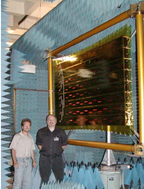
Figure 4 – The membrane waveguide array antenna in GTRI’s near-field range. Pictured with the array are Leo Lichodziejewski (right) of L’Garde, Inc., the fabricator of the array, and Glenn Hopkins (left) of GTRI.
