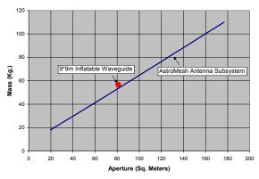
Figure 12. Waveguide Mass Comparisons
