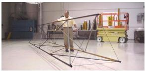
Figure 7. Sub-Tg 8m Rigidizable Space Truss
