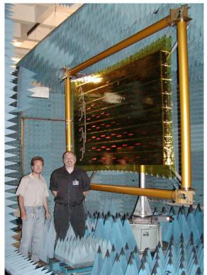
Figure 2. Waveguide Array in GTRI Near-Field Test Range
