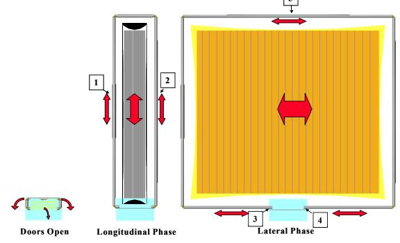
Figure 11. Waveguide Deployment Sequence
