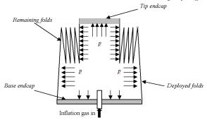
Figure 8. Conical Inflation Schematic
