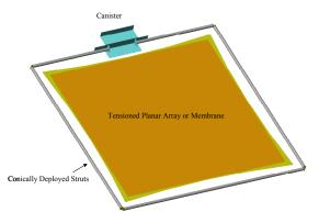
Figure 3. Optimized 9m\*9m Radiometer Array
