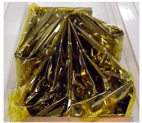
Figure 6. Packaged Waveguide Array
