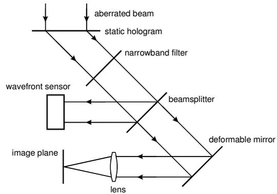
Fig. 7B. Hybrid holographic correction. The large scale aberrations are removed by a static hologram, while minor temporal changes in the mirror are corrected by the small-stroke deformable mirror.
