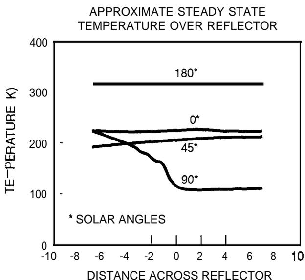
Fig. 9. Reflector Orbital Temperatures
