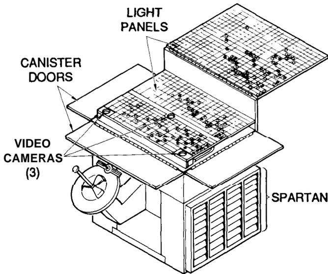
Fig. 5. Canister and Spartan
