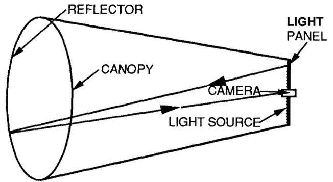
Fig. 6. Surface Measurement System Configuration (Not to Scale)
