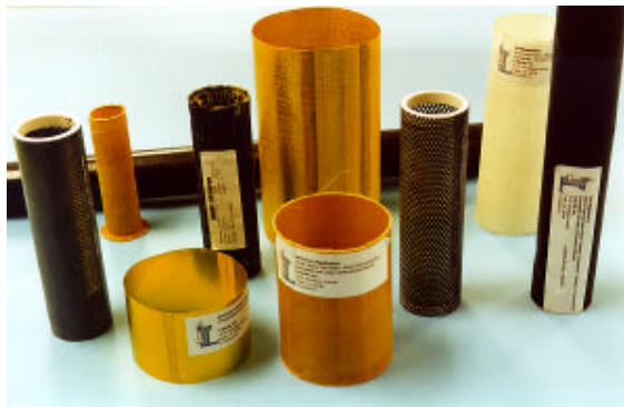
Figure 6. Rigidization Technologies Used by L'Garde
