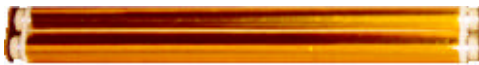
Figure 7. Aluminum Laminate Bundled Tubes 1.7X better bending buckling than equivalent mass tube 2.5X higher short compressive strength
