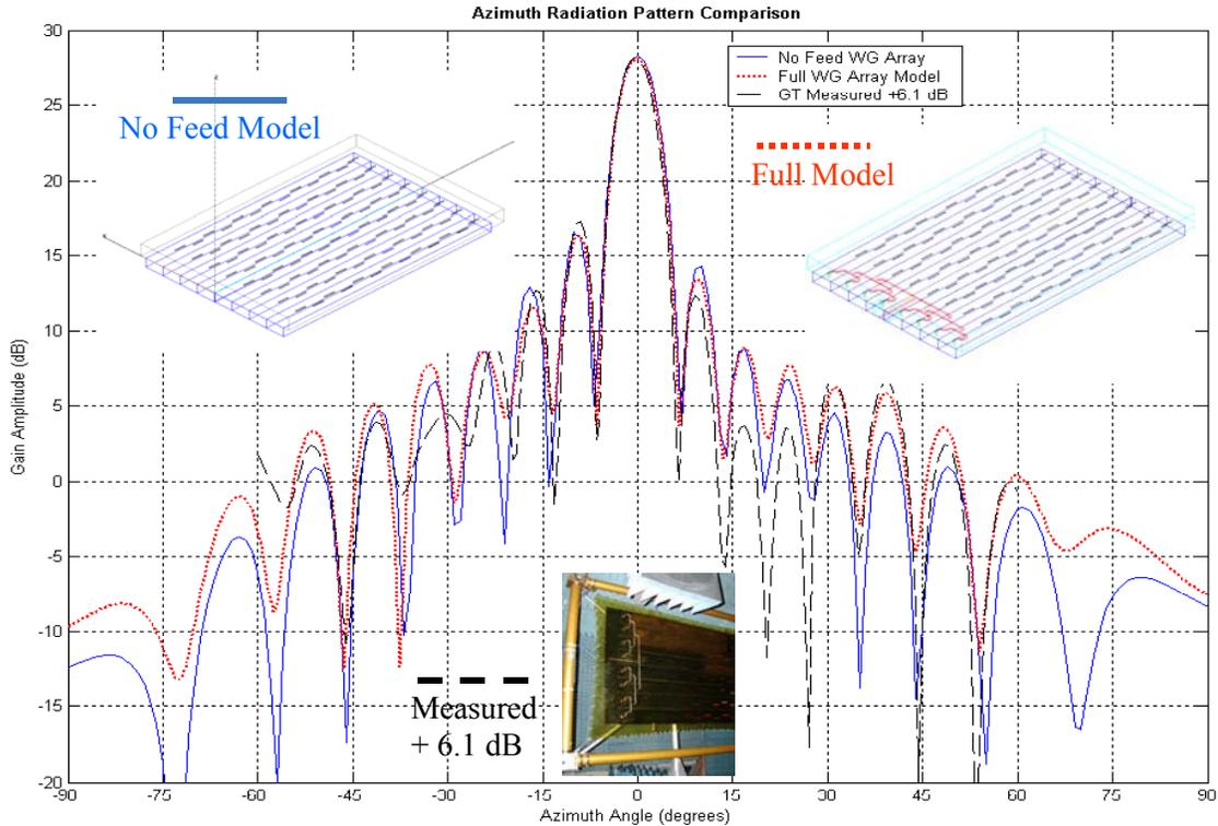
**Figure 5 – An overlay of H-plane far field radiation patterns from: the simulated array with no microstrip beam former (blue, solid), the simulated array with beam former (red,dotted), and measured data corrected in gain to match the simulated levels (black, dashed).**
