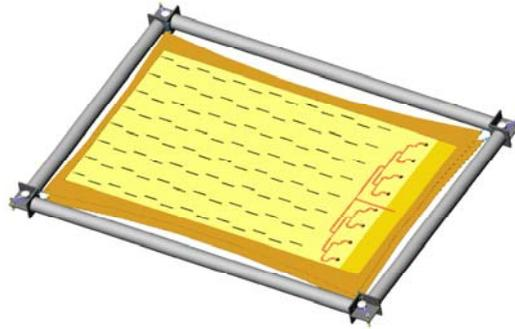
**Figure 1 – CAD model of the waveguide array**
