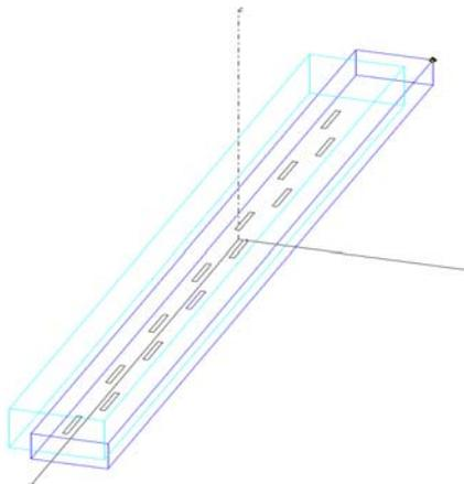
**Figure 2 - FEM model of one waveguide linear array**
