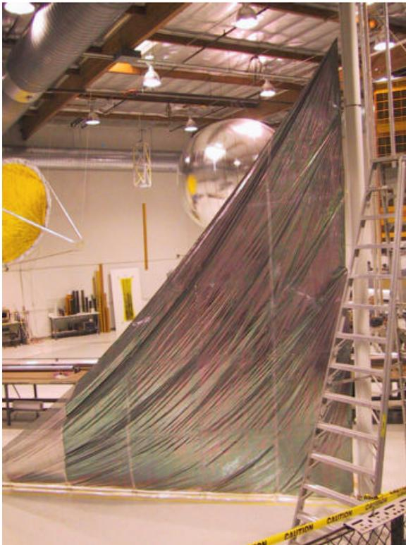
Figure 10. Mylar Sail During Deployment Test
