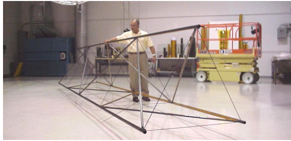
Figure 7. Sub-Tg 8m Rigidizable Space Truss
