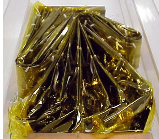
Figure 6. Packaged Waveguide Array
