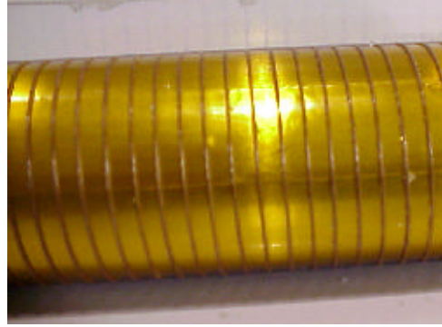
Figure 6. Reinforcing PBO Filament
